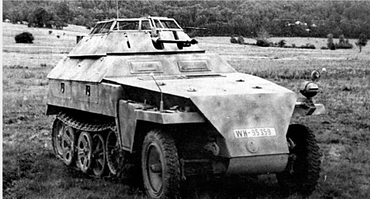
An Sd.Kfz.250/9 with a turret mounting a 20mm gun.
