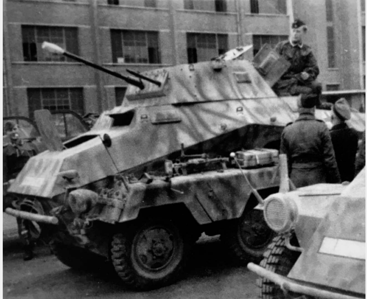
An Sd.Kfz.232 reconnaissance armoured car with an extended-range radio, as issued to the 1st Company.
