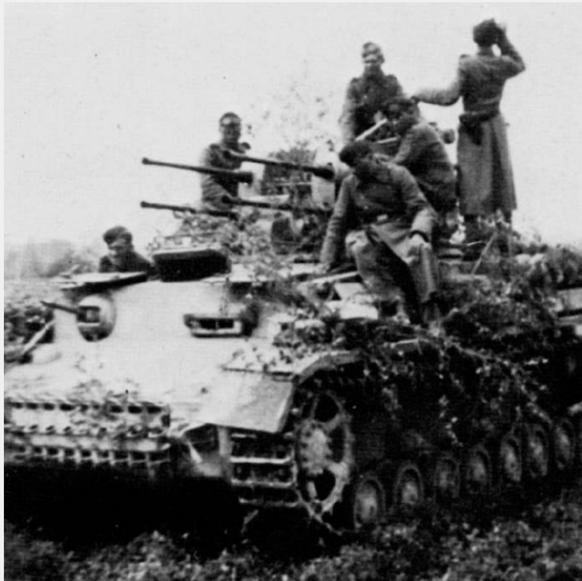
The 20mm Flakvierling on the hull of an early Mark IV Panzer.
