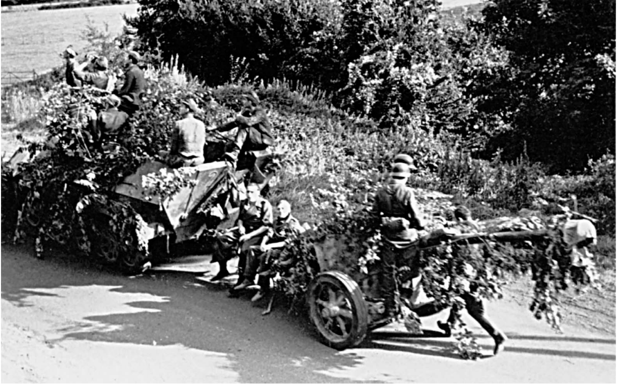
A Hanomag halftrack towing a 75mm Pak 40 anti-tank gun. Note how 'air conscious' the crew are.
