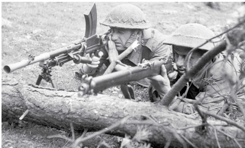
The Bren gun was a light machine gun developed as an accurate weapon that would not squander ammunition. Rate of fire was low, at 500–520rd/min, and the magazine held 30 rounds. Effective range was 550m. Every soldier in the section carried two magazines for the weapon. Here, soldiers with a Bren gun are pictured on exercise in 1943. (Lieut. C.E. Nye / Canada. Dept. of National Defence / Library and Archives Canada / PA-141308)
