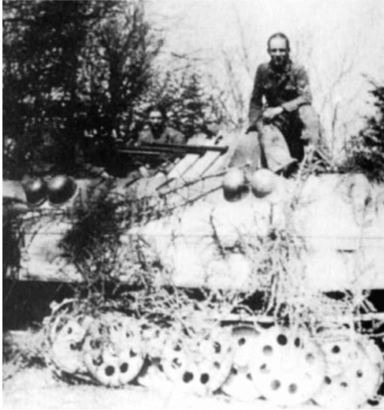
Armored personnel carrier of 3rd Battalion of SS Panzergrenadierregiment 26 with 2 cm three-barreled gun (aircraft cannon).
