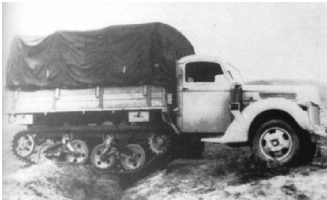
Two-ton “Maultier” half-track truck, Model Ford, used as a tractor for 3.7 Flak of 4th Battery of SS Flak Battalion 12, in place of the unavailable self-propelled chassis.
