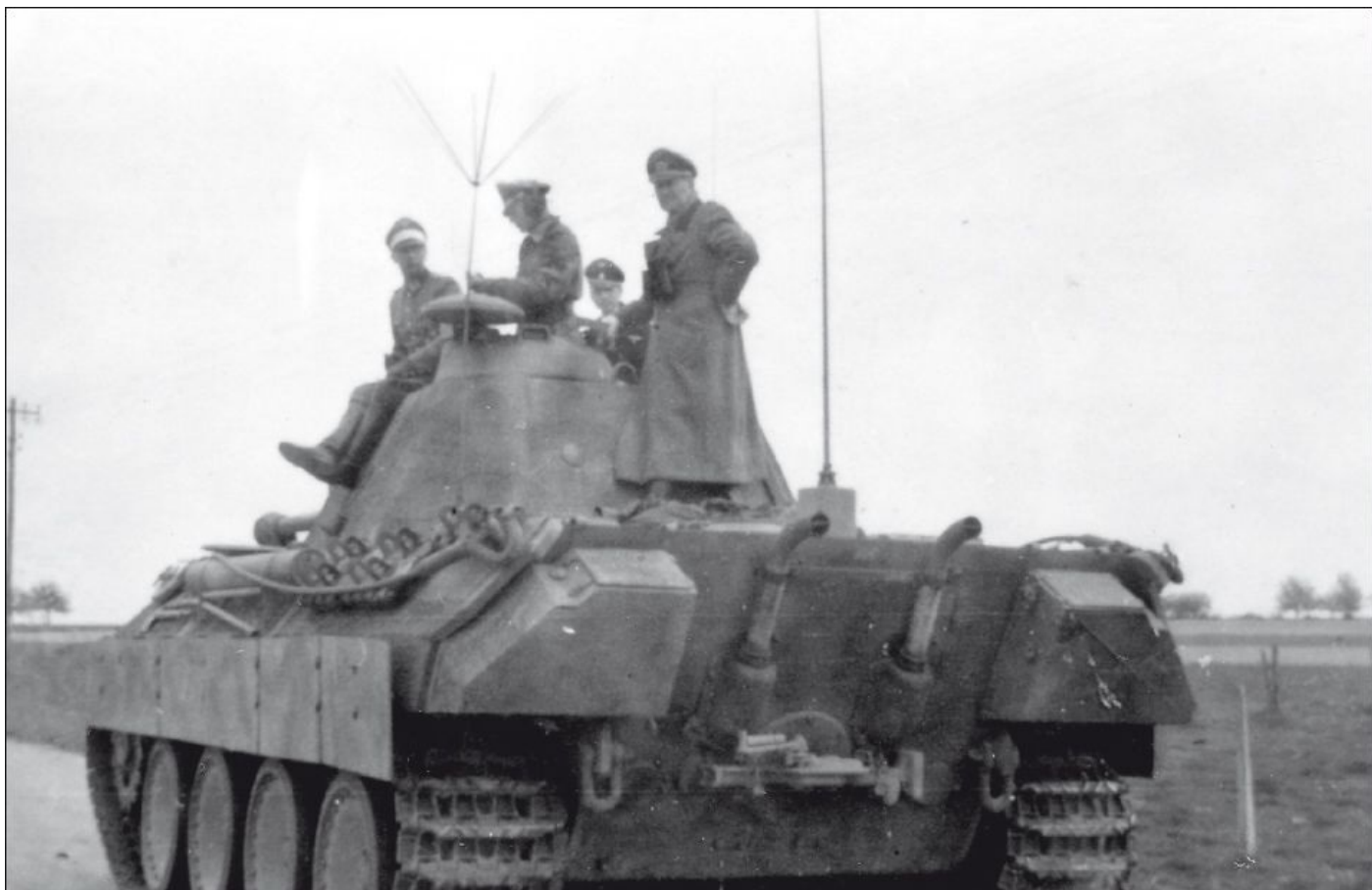
Obersturmbannführer Max Wünsche in his Panther command tank ( Pz Bef Wg Panther ) during an exercise with SS-Panzer Regiment 12 in Belgium, March 1944. The additional antennae for the command equipment are clearly visible. (National Archives)
