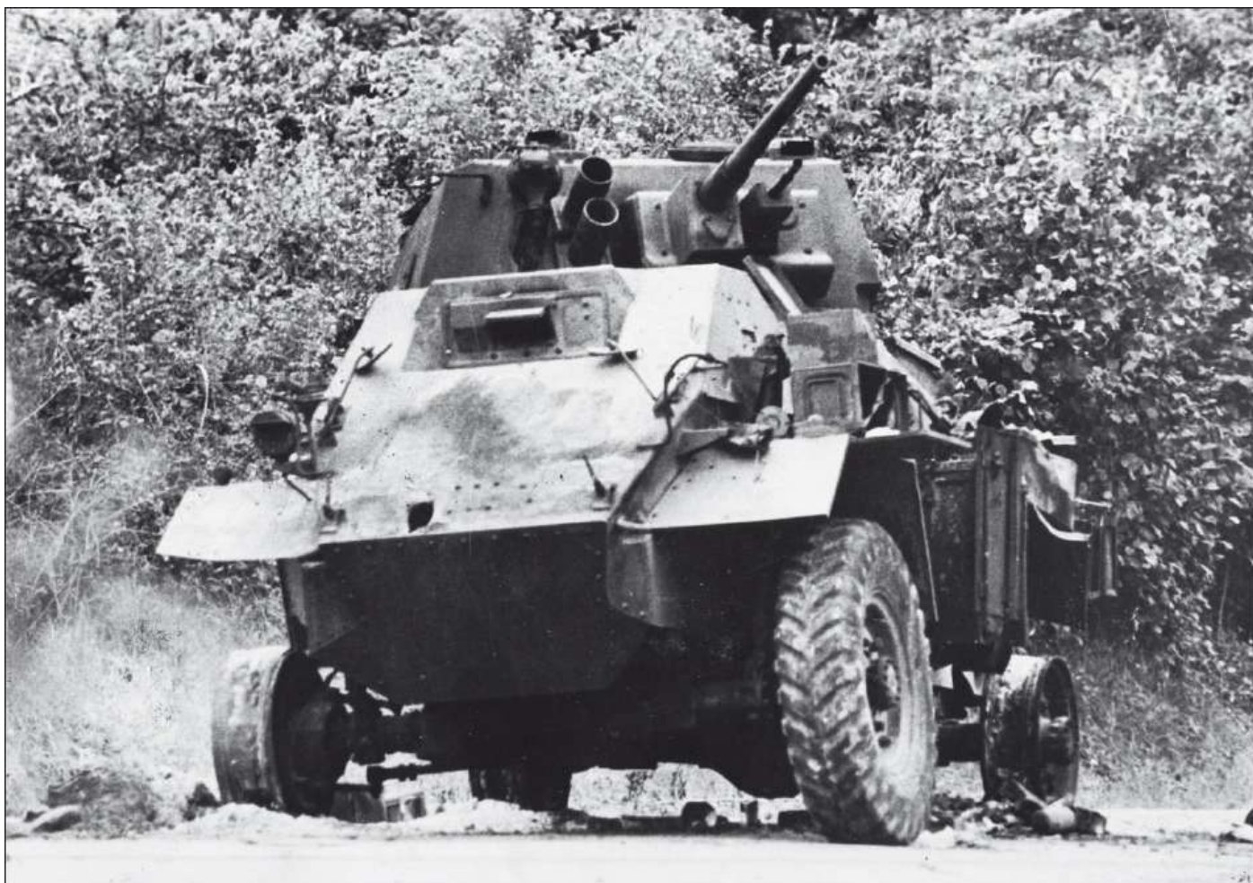
A knocked out British Humber Mk. IV armoured reconnaissance car near Caen in June 1944. The armament of this 6.5 ton vehicle consisted of a 37 mm gun and a coaxial machine gun. Its crew of three was protected by a maximum 15mm armour. The vehicle was mainly used by the reconnaissance regiments of the British infantry divisions. (Hungarian Institute and Museum of Military History 52809)
