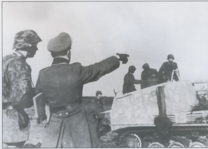
A 'Wespe' self-propelled howitzer from I./SS-Panzer-Artillerie-Regiment 12 prepares to fire during the training exercise directed by the battery commander. There were two batteries of 'Wespe', mounting the 10.5cm leFH18 howitzer, in the battalion and one battery of 'Hummel' which mounted the 15cm sFH18 howitzer. The vehicle is painted in overall dark yellow with a camouflage pattern of green and brown lines sprayed over.
