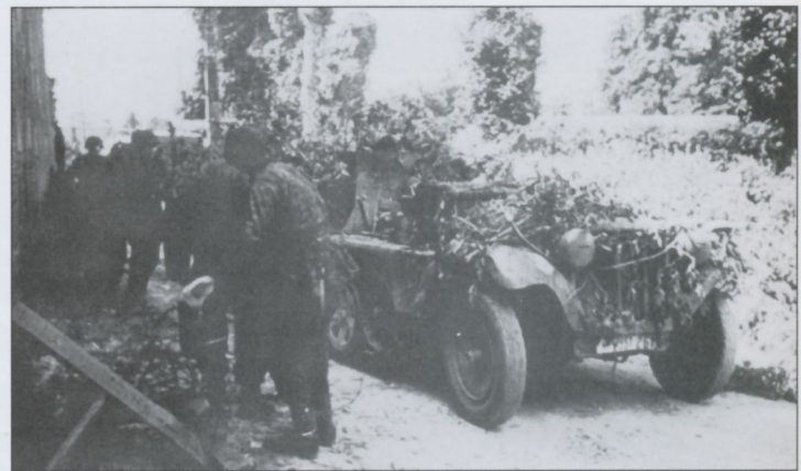
Three photos showing a 15cm sIG33 from 13.Kompanie, SS-Panzer-Grenadier-Regiment 25 being towed into the abbey compound by an Sd.Kfz.10 half-track prime mover. Each battalion in SS-Panzer-Grenadier-Regiment 25 and 26 were equipped with a battery of six towed 15cm sIG33 howitzers. The divisional emblem can be seen on the right mudguard of the half-track.
