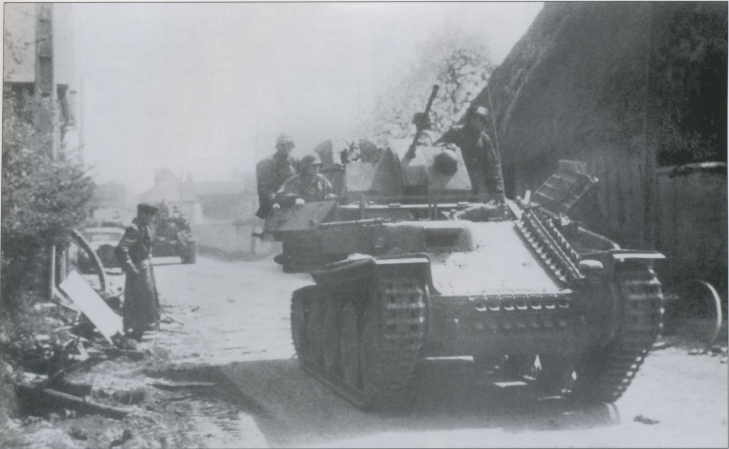
A column of 2cm Flakpanzer 38(t) Ausf.L (Sd.Kfz.140) from SS-Flak-Abteilung 12 in the Caen area, early June 1944. There were 140 of these Flakpanzers built on the chassis of the obsolete Pz.Kpfw.38(t) from November 1943 to February 1944, armed with the 2cm FlaK38 anti-aircraft gun. They were issued to the Panzer divisions in January and February 1944, including eight to SS-Flak-Abteilung 12.
