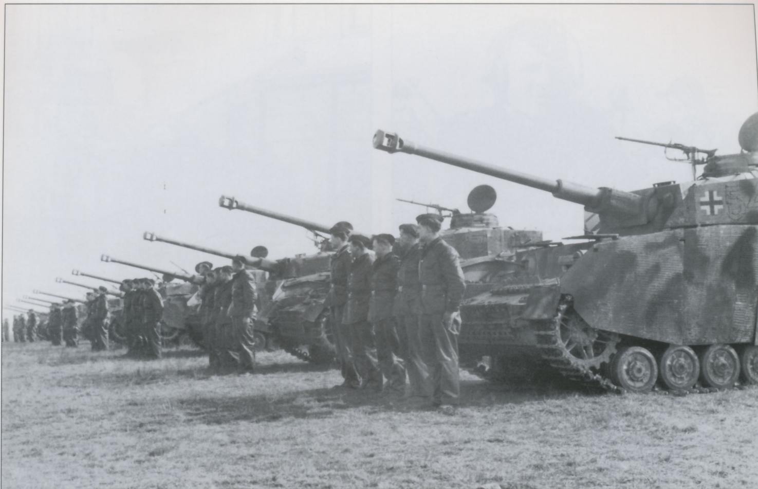
Here, the crews from 5.Kompanie of II./SS-Panzer-Regiment 12 line up in front of their new Pz.Kpfw.IV Ausf.H for inspection. The vehicles are painted in overall dark yellow and have a camouflage scheme of green and red-brown patches sprayed randomly over. A coat of Zimmerit anti-magnetic mine paste has also been applied at the factory to the turret and hull side skirts (Schürzen). At this time, the three digit tactical numbers were painted in a black stenciled outline. All members of the crew are wearing the black leather Kriegsmarine U-Boat jacket and trousers which had been originally provided to the Italian Navy. They had been brought back to Germany by 1.SS-Panzer-Division 'Leibstandarte' in the fall of 1943 after Mussolini had been deposed.
