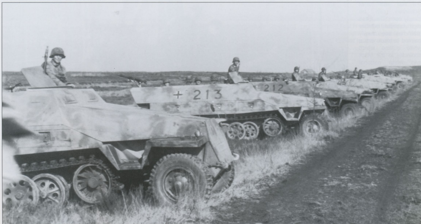
A row of new Sd.Kfz.251/1 Ausf.D armored half-track personnel carriers from III./SS-Panzer-Grenadier-Regiment 26 during von Rundstedt's inspection. These vehicles are also painted in overall dark yellow with a camouflage scheme of green and red-brown patches. The three digit tactical numbers are painted in solid black.
