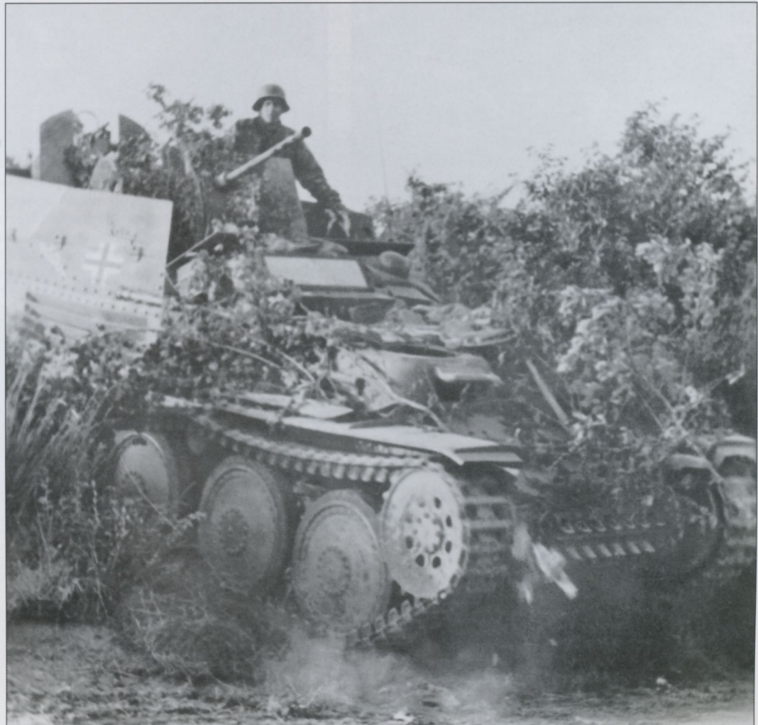
Another 2cm Flakpanzer 38(t) Ausf.L drives out of a field and onto a road. The hinged armor shields are raised up revealing a national cross that is painted on the side of the plates. (M. Bayerl)
